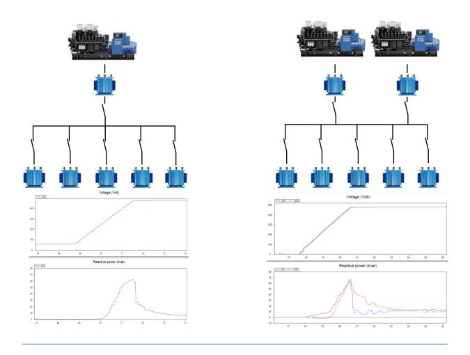
1.2 Synchronizing as many generators as possible in less than 15 seconds
