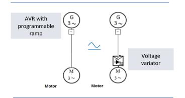
Dead bus synchronizing is similar to starting with a soft starter with a fixed frequency (generator frequency) and a voltage ramp provided by the voltage regulator. The current impact on the generator is much lower than for direct starting with nominal voltage.
