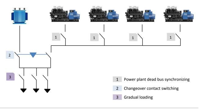
On large-scale power plants, live bus synchronizing can take too much time. Indeed, the conventional live bus synchronizing technique for several generators in parallel involves production equipment deployment time which is difficult to reduce.
