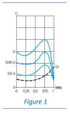
Figure 1 shows the torque/speed characteristics for an asynchronous machine depending on the voltage supply.
